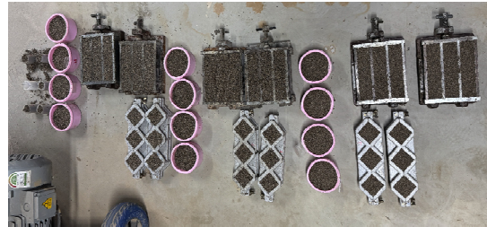
Fig. 4. (Color available online) Mortar specimens prepared for testing.
