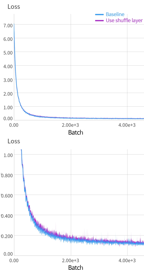
Fig. 4. (Color available online) CCE loss trend according to the application of segment unit shuffle layer.
