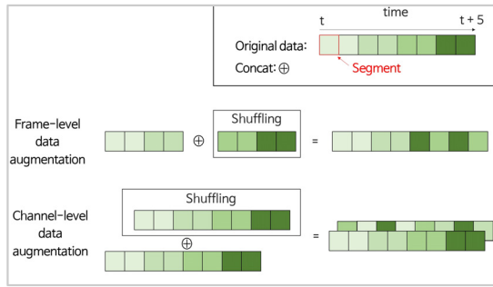
Fig. 5. (Color available online) Augmentation strategy for frame-level data augmentation and channel-level data augmentation.
