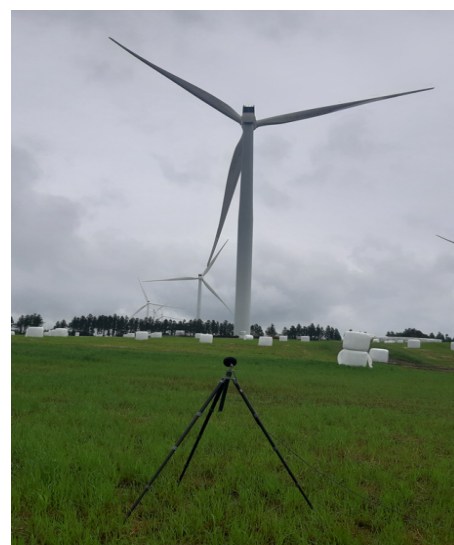
Fig. 3. (Color available online) Wind turbine noise measurement photograph.
